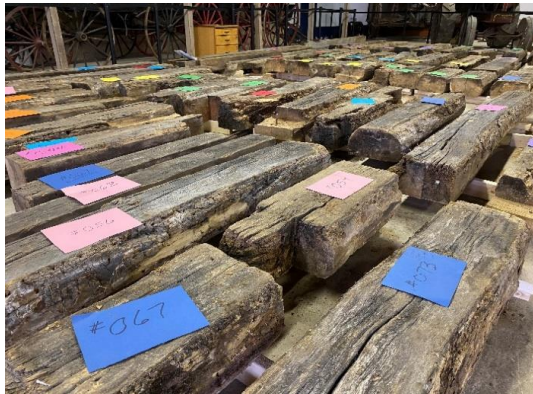
Figure 3 – In January 2024, contractors began the task of sorting, inventorying and assessing the loose logs for reconstruction. At that time, it was determined that a number of logs were too deteriorated to be used in the reconstructed building. Timber was obtained from deconstructed log homes and barns of a similar age from around the County so that they could be seamlessly integrated into the cabin reconstruction.
